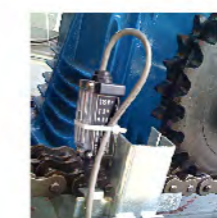
驱动链断裂保护 Drive-chain breaking protection
